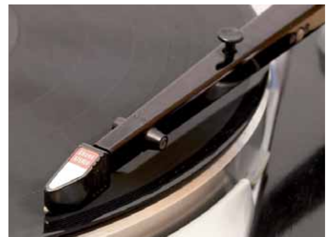
Top: tonearm pillar with counterweight Bottom: vertically moving part of the tonearm with its delicate head
